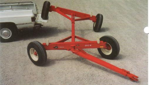
E-Z Trail wagons flex their muscles over terraces and through waterways! There is no terrain too rugged for the triple torsion telescopic reach that stretches from 7' to 15' by fractional increments. The reach bolts can't wear and the "can't slip" clamp is tested up to 16,000 lbs. of drawbar pull. U.S. Patent No. 5,042,831.
