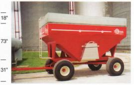
500 Bu. 8-1/2' x 14' on 1584 16.5L x 16.1 tires. Inside extension flanges are self cleaning. US Patent #4,460,214. All wagons have adequate chute height, 17" to 21", for unloading into auger hoppers.
