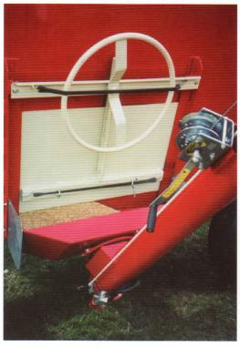
2, 3, or 4 compartments can separate seed varieties or fertilizer. To easily open any compartment, simply insert a pin thru the main door and the inner door of any or all compartments. U.S. Patent #4,646,942.
