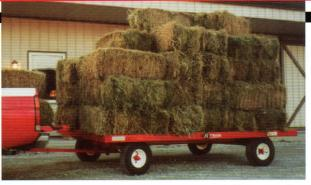
6' x 10' Jr. Flat Rack has 2" treated floor on 3 x 6 sills and is framed all around in steel with stake pockets. Its low 21" deck height makes loading E-Z. It can haul up to 50 bales and is very useful in orchards and nurseries, for landscaping and displays. Narrower widths are also available for vineyards, and factory in plant use.
