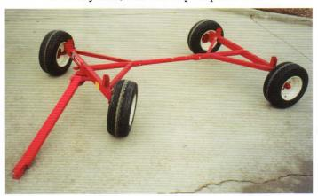
Jr. running gears have a 2 ton capacity and are available in 46" or 60" wheel tread. 5.70-8 tires are standard, shown here with optional 20.5 x 8-10 tires.
