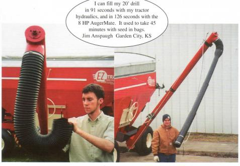
The 4ft. flex spout is corrosion resistant & highly flexible. By turning the end into a "J", you can "hop" from one hopper to the next without turning the auger off.
