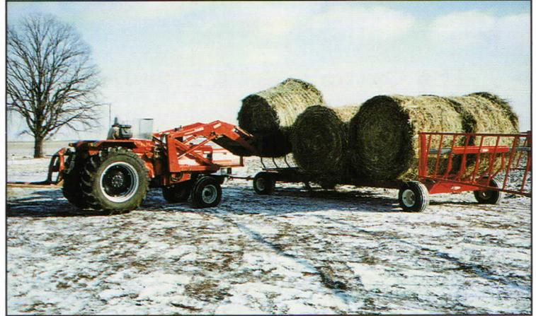
Low profile 1200 x 12, 10 ply flotation tires for low comfortable feeding. Panels swing open for loading with 3 point hitch or front loader.
