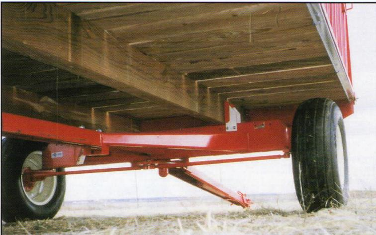
E-Z Trail floors are designed lower, lighter, stronger, & longer lasting. The 2 x 8 floor boards and 4 x 8 sills are made of Southern Yellow Pine treated for long life. The special cut sills are 27% stronger than commonly used 6 x 6 sills, according to the the University of Wisconsin Forestry Dept. The floor is framed all around in steel for added strength and warp prevention. Since there are fewer collection points for residues which cause wood decay, floors will stay cleaner and last longer.
