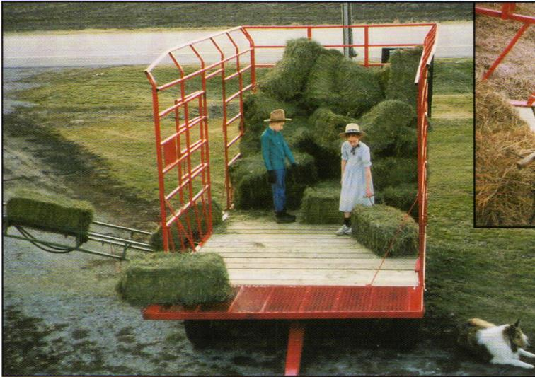
The front gate & side doors are mounted flush to the floor & made of flattened expanded metal which provides a smooth "slide" exit for unloading heavy bales **without** lifting.
