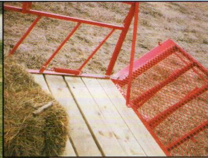
The "see-thru" front gate is E-Z to open with its pressure release latch & EZ lift spring. It serves as a solid platform to begin unloading. Bales unload easier starting at the front, then unloading the rear half thru the side doors. It's called "LIFO," last in first out. However, rear swing gates are available as an option.
