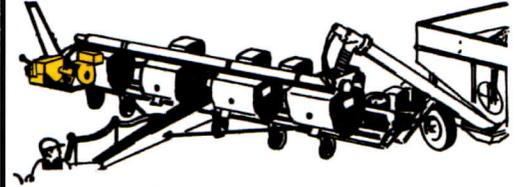
Can be direct mounted on drill or planter to run fill augers.
