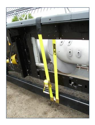
Storage tray fits into front end of top rail. Tighten handle nut to secure.
