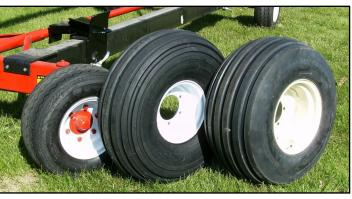
Standard tires for 21'-31': Low profile 20.5x8-10 E Range 10 ply Optional: 9.00-10 flotation tire
