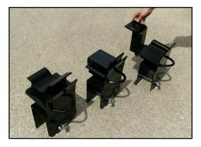
Patented two-way slider brackets can be easily adjusted to accommodate any brand of grain or corn head. Brackets are designed to fit round or square frames & channels.
