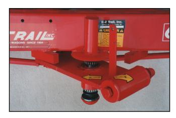
"Lifetime" accurate trailing is assured by E-Z Trail's original steering centered around sealed tapered roller bearings, truck type ball joints and dual stops with 100% greater oversteer protection. All steering parts are weather protected for lifetime outdoor use.
