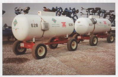
Model 860 has 16,000# capacity and 60" wheel tread which is ideal for side dressing 30" rows.
