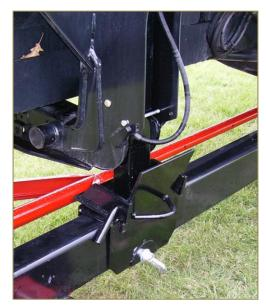
Head fastens to hauler bracket by inserting pin through sleeve on leg bottom. (Fig. 3) Riser brackets can be positioned on center of lower rail if needed to support the combine adapter.
