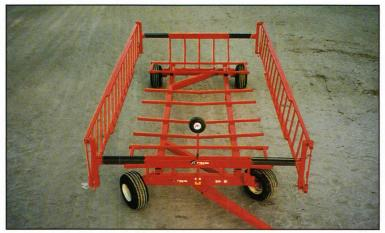
Here it is! A big bale carrier with quick attach 32 ft. feeder panels! Side panels slide out to 11 ft. wide and swing open for EZ loading.
