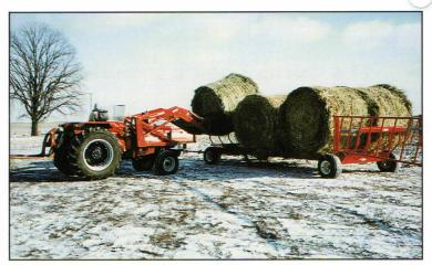
Low profile 1200 x 12, 10 ply flotation tires for low comfortable feeding. Panels swing open for loading with 3 point hitch or front loader.
