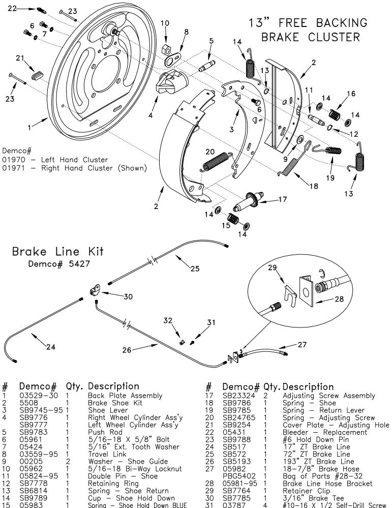
Spring - Shoe Hold Down BLUE SB9790 Spring - Shoe Hold Down MAROON
